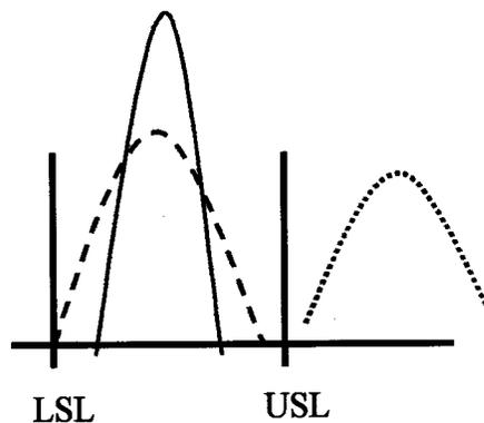
If the process is centered within the specs, and is approximately “normal” then  $C_p = 1.00$  results in a fraction non-conforming (f.n.c.) of 0.27%. Note that  $C_p=1.00$  doesn’t guarantee that there will be only 0.27% non-conforming product. What it does guarantee is that, assuming normality, a stable process centered with respect to the specs, and the correct value of  $\sigma$ , there will not be less than 0.27% of non-conforming product.
