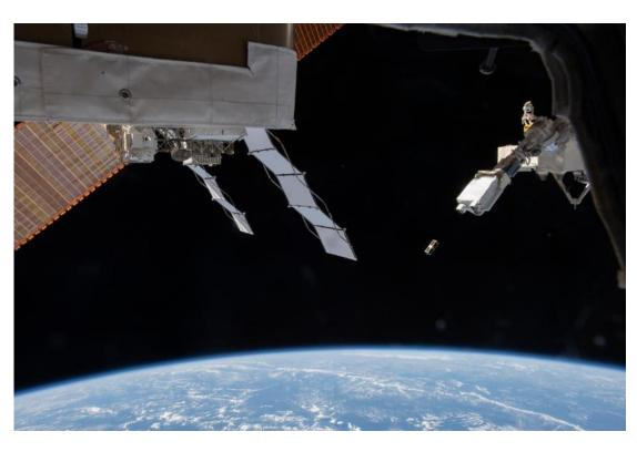
An external view of the deployment of the AQT-D CubeSat from the JEM Small Satellite Orbital Deployer aboard the International Space Station (ISS). AQua Thruster-Demonstrator (AQT-D) is a 3U CubeSat demonstration of a water resistojet propulsion system developed by The University of Tokyo.
