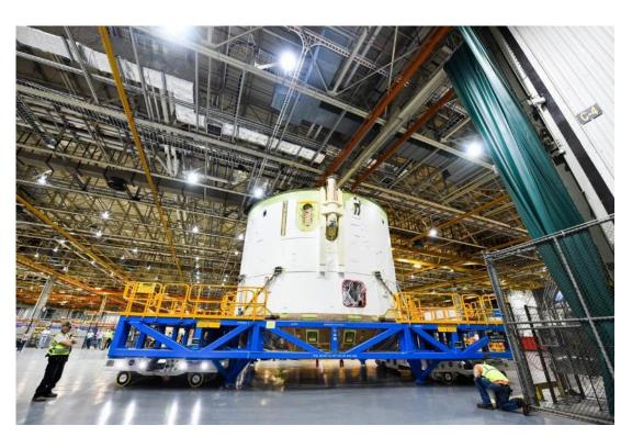
Technicians at NASA's Michoud Assembly Facility in New Orleans moved the engine section for NASA's Space Launch System (SLS) rocket to another part of the facility on Sept. 3 to prepare it for joining to the rest of the rocket's core stage. The engine section, which comprises the lowest portion of the 212-foot-tall stage, is the last major component to be horizontally integrated to the core stage.
