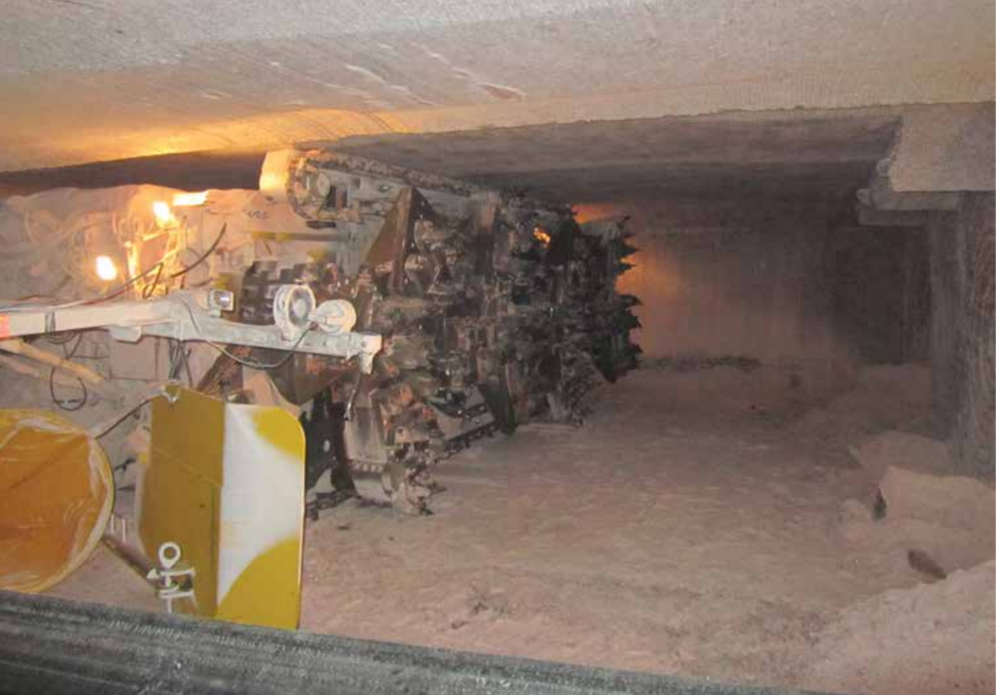
AN EXAMPLE OF an underground mining machine used to cut soft rock, or ore, at the Mosaic Potash Colonsay mine site in Saskatchewan, Canada.
