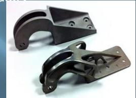
3D printed jet engine part is 50% lighter
