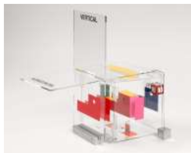
Fig. 2: Using a projection box in the 3 rd quadrant to see the object projected from different sides.
