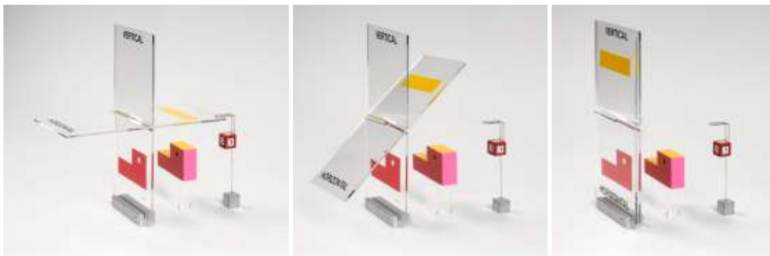
Fig. 1: Principles in creating two basic views (Top and Front), using 3 rd angle orthographic method.
