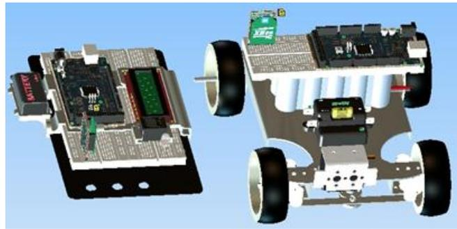
**Figure 3.7: Computer Models for the Remote Control Unit and the CDR**
