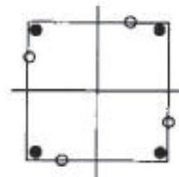
Figure 5. 2 2 Factorial Design with Two Levels per Factor (●) Rotated (○) to Have Four Levels per Factor
