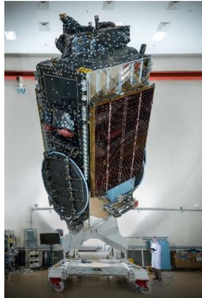
Jupiter 2 / Echostar XIX; highest throughput satellite (greater than 200 Gbps) on-orbit. Launched in 2016.
